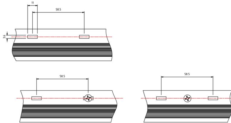
3. When installing horizontally, general consideration is given to good practice and proper drainage, hence the perforated section that runs adjacent to the underlock of the cladding sheet is installed as the top of the sheet.
