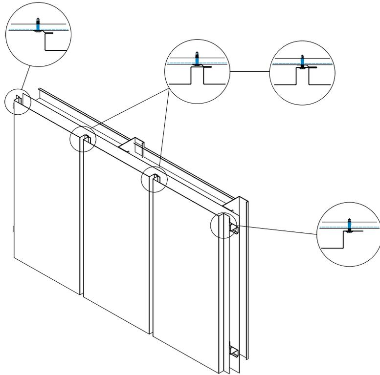
When installing horizontally, general consideration is given to good practice and proper drainage, hence it is desirable to install the cladding sheet with the under-lock tab facing downwards. To facilitate this, cladding sheets can be installed from top to bottom. This technique also allows for the fixing fastener to be concealed.
