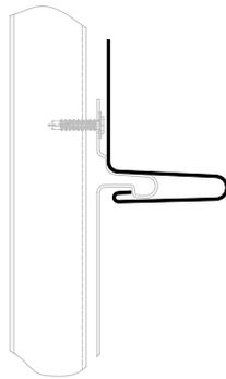
4. Align panel over and under lap ribs and apply horizontal pressure.
