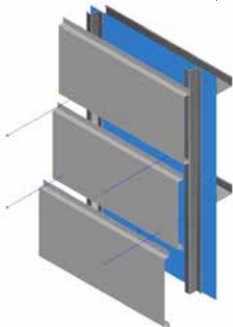
The alternate technique of installing from the bottom up will result in either poor drainage detail or having to fasten the fixing through the express joint which exposes the fastener screw and results in restricting movement of the cladding, which are generally considered undesirable and not recommended.
