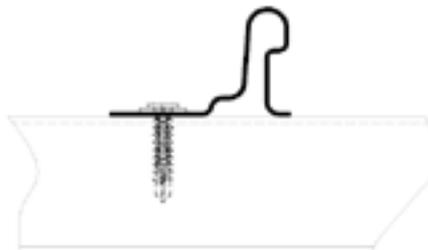
Take care to place the screws in the centre of the slotted holes to allow for expansion and contraction, however it is not always possible or practical to do so. Screws can be placed either through the slotted holes or directly through the sheet. Where screws are fitted directly through the sheet tab and where aesthetics are important, it is advisable to pre-drill an oversized hole to accommodative thermal movement of the sheet.
