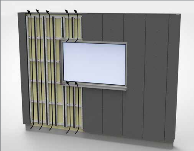
FIGURE 2. Ventilation air flow
