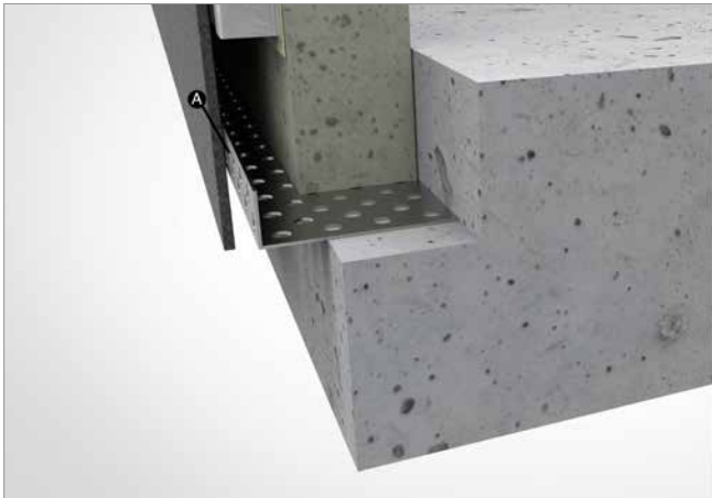
FIGURE 14. A. Anti-vermin perforated angle to sit flush against façade board
