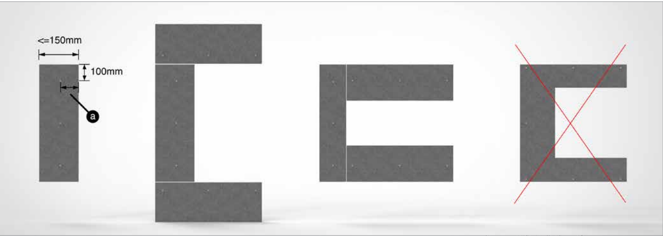
FIGURE 21. Correct installation of Genesis Signature façade boards at windows, doors and openings a: If the small cut-outs are not wider than 150mm, they can be mounted with only one rivet in the middle of the board.
