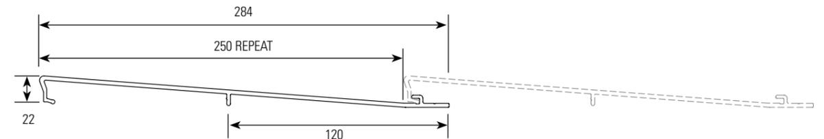
Thickness: 2.8mm    Weight: 9.37kg/m<sup>2</sup>    Length: 6.5m    Effective Cover: 250mm per panel
