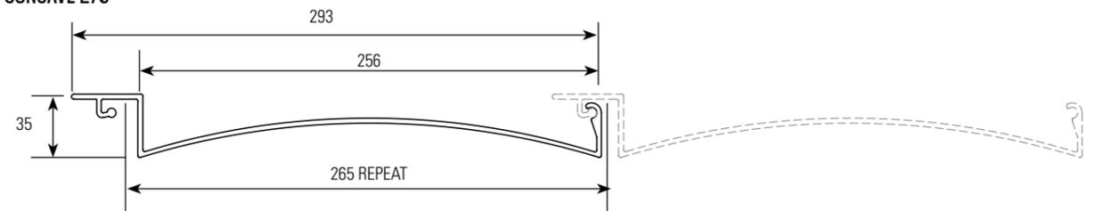
Thickness: 2.8mm    Weight: 10.38kg/m<sup>2</sup>    Length: 6.5m    Effective Cover: 265.2mm per panel
