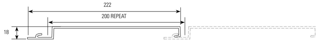
Thickness: 2.5mm      Weight: 8.82kg/m<sup>2</sup>      Length: 6.5m      Effective Cover: 200mm per panel
