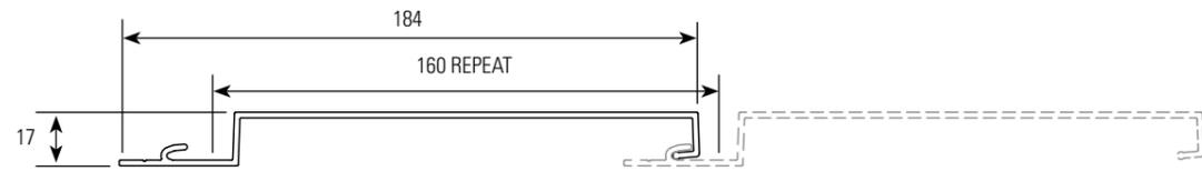
Thickness: 1.8mm      Weight: 6.9kg/m<sup>2</sup>      Length: 6.5m      Effective Cover: 160mm per panel
