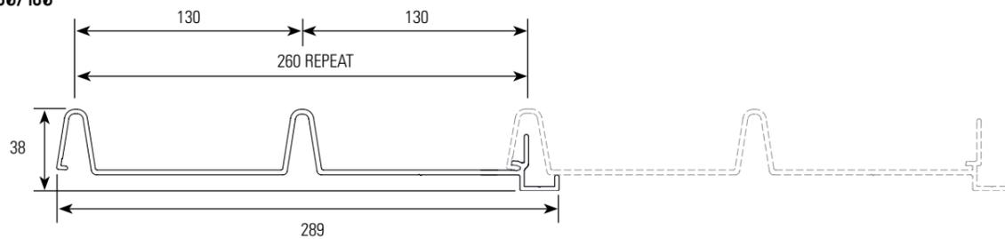
Thickness: 2.8mm    Weight: 12.69kg/m<sup>2</sup>    Length: 6.5m    Effective Cover: 260mm per panel
