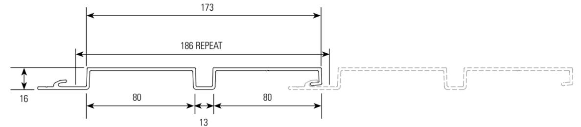
Thickness: 2mm      Weight: 8.11kg/m<sup>2</sup>      Length: 6.5m      Effective Cover: 186.1mm per panel
