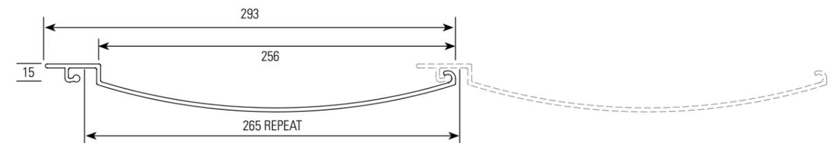
Thickness: 2.8mm    Weight: 9.64kg/m<sup>2</sup>    Length: 6.5m    Effective Cover: 265.2mm per panel
