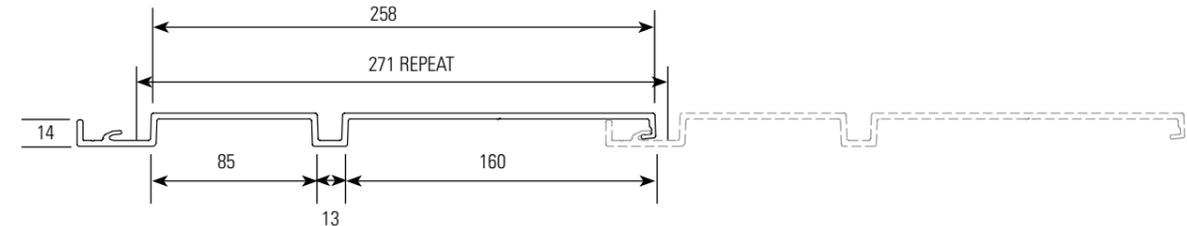
Thickness: 3mm      Weight: 10.94kg/m<sup>2</sup>      Length: 6.5m      Effective Cover: 271.1mm per panel
