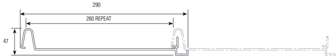
Thickness: 2.8mm    Weight: 11.07kg/m<sup>2</sup>    Length: 6.5m    Effective Cover: 260mm per panel
