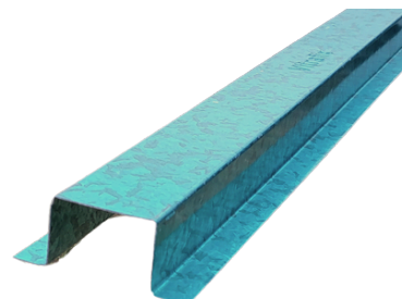
Steel Top Hat 35mm 0.75BMT 50x35 5.8m
