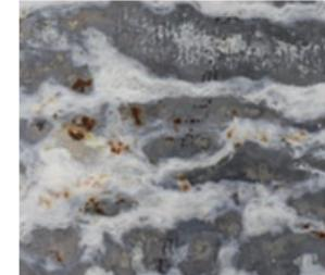
Z275 after 1000hrs of salt spray exposure.
